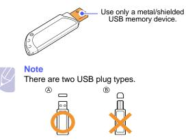
Insert an USB memory device into the USB memory port on the side of your machine.
